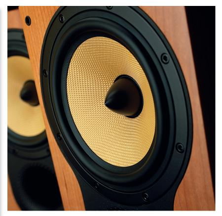
■ 165mm cast frame main driver, equipped with a 120mm woven Kevlar/polymer cone. The magnetic motor features the latest 'Balanced Drive' metalwork to minimise distortion, and a larger magnet than before, while magnetic shielding is no longer used here. A bullet-shaped phase-compensating dust dome covers the voice coil, and is now part of the cone rather than the pole piece, increasing the radiating area and avoiding chuffing sounds.
